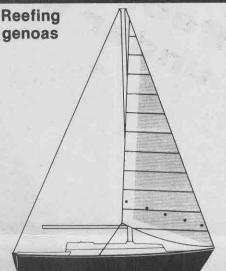
A simple and inexpensive way to reduce headsail area is to reef the sail in a manner similar to the mainsail. However, care and consideration must be given as to whether the cloth weight can handle the increased strain of stronger winds. While Fogh Sails recommends that you select sails designed for a given range of conditions rather to extend one sail's use into conditions of higher strains, they can offer valuable advise on reefing systems for headsails.
